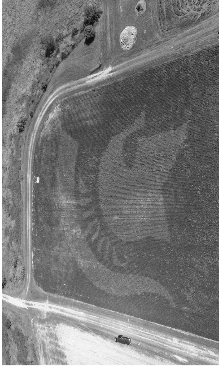
MSU campus field planted with light and dark soybean varieties using GPS guided precision planting.
