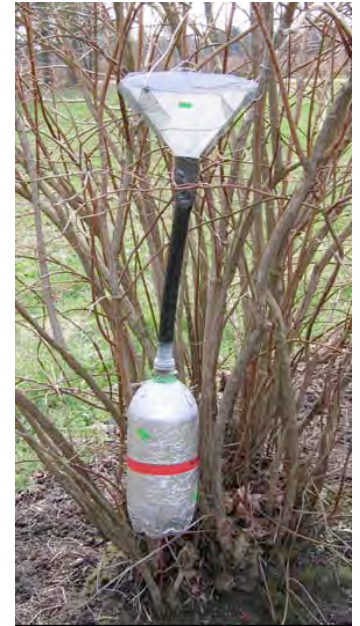
Figure 3. Michigan State University spore trap (Sporomatic 2000 Deluxe) designed to collect rain water and spores of rain-splash-dispersed fungi. The aluminum foil is to protect the sample from heating up due to sunlight.
