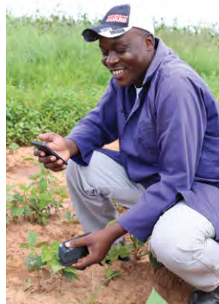
Taking measurements using the MultispeQ and a mobile phone.
