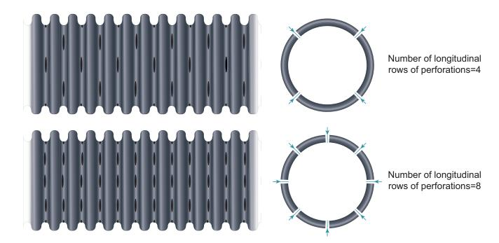
Figure 1- Top: A staggered regular-perforated pipe with 4 perforation rows per valley, rotated 45 degrees every other valley. Bottom: A non-staggered regular-perforated pipe with 8 perforation rows per valley.
