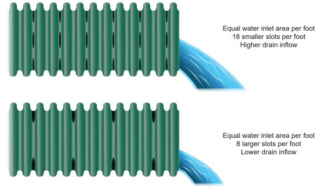
Figure 4- The pipe with the greater subdivision of openings has a higher drain inflow. Greater subdivision of openings can be achieved by increasing the number of perforation rows.
