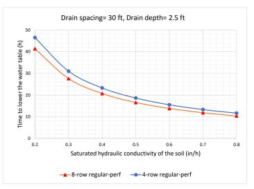
Figure 3- An 8-row regular-perforated pipe lowers the water table from the soil surface to 1-ft depth, 11% more quickly than a 4-row pipe, when installed at 30-ft spacing and 2.5-ft depth. Drainable porosity is 0.04 and depth to restrictive layer is 6.5 ft.
