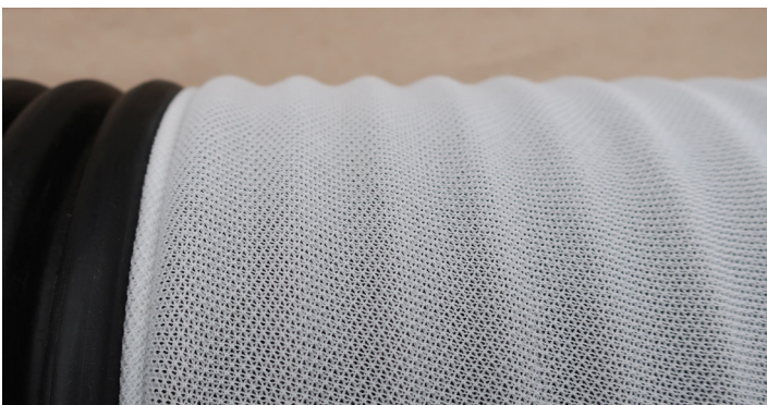
Figure 6- Top: A photo of a sand-slot pipe. Bottom: A photo of a knitted-sock envelope wrapped around a regular-perforated pipe.
