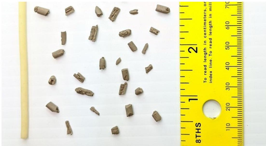
Figure 7- Barrel-shape soil crumbles made during the rolling process. During the rolling process, if the thread crumbles into barrel-shape pieces before reaching the 1/8" diameter, the soil is dry enough for moling. The item on the left is a bucatini pasta with a 1/8" diameter after soaking in water, which can be used as a reference for the desired 1/8" diameter (photo credit: Zouheir Massri).
