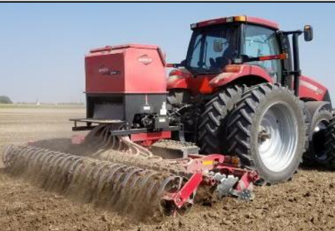
Broadcast Incorporation- BI: Horsch Joker with Gandy Air Seeder, Degelman Pro Till, Vertical Tillage Tool
