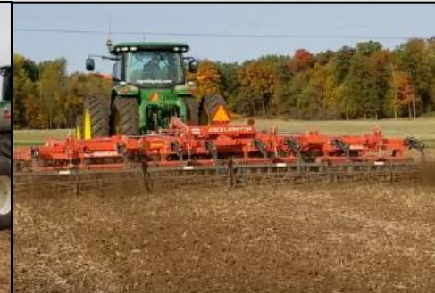
Broadcast Incorporation- BI: Horsch Joker with Gandy Air Seeder, Degelman Pro Till, Vertical Tillage Tool
